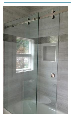
Durable stainless steel construction • Available in polished chrome, brushed steel, and matte black finish • Accomodates glass thicknesses from 5/16" to 3/8" • 4 ball bearing wheel provided security and smooth quiet operation • Maximum door size of 30" • All installation hardware included except clamps or channel for fixed panel • Fixed and gliding panel are reversible • Maximum weight of 88 lbs
